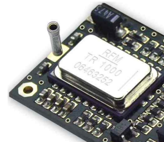
K option: with a small connector for the AN-xxx-03 antenna (1/4 whip)
