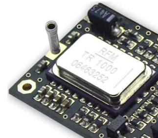
K option: with a small connector for the AN-03 antenna ( \frac{1}{4} whip)
